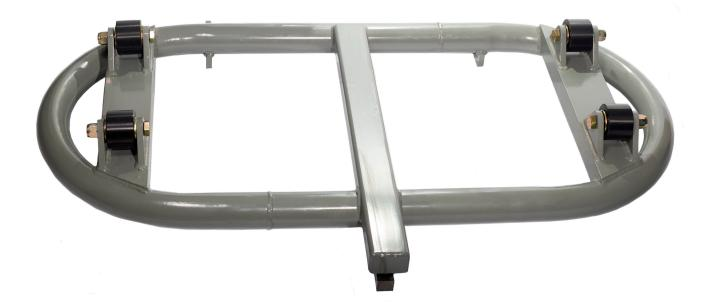
The JCS Model 4710 Electronic Ton Cylinder Scale is designed for years of safe, continuous use for weighing 2,000 pound compressed cylinders. The low profile 2.5" Epoxy coated tubular steel frame coupled with UHMW poly-ethylene rollers allows for positioning and rotating the container with ease. The rolled tubular design eliminates angular edge hazards.
