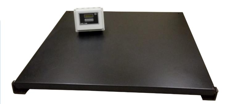
The JCS Model 4720 Electronic Platform Scale is designed for years of safe, continuous use for weighing 8,000 pound compressed cylinders. The low profile 3" Stainless Steel platform is protected by a textured Polane finish. The load cells, leveling feet, and hardware are all stainless steel. There are four standard sizes plus customizable versions available.
